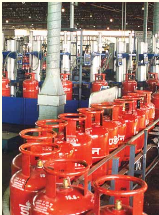
Indane bottling Plant at Madanpur Khadar near Delhi – one of the 89 plants, which together roll out 12.3 lakh cylinders per day.
